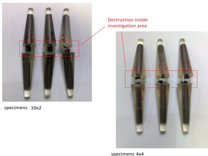
Fig. 18 Photo of specimens after compression
